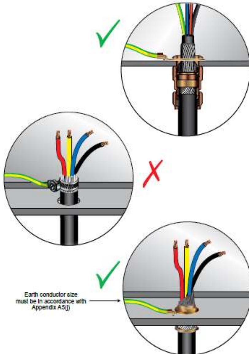
**Note: all glands should be mechanically and electrically sound, secured and tightened using the appropriate tools**
