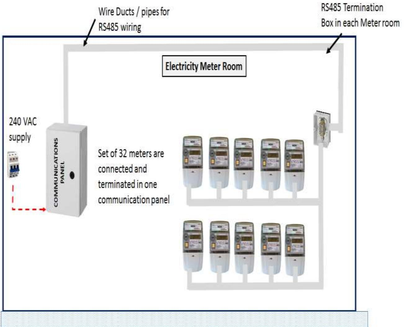
**Appendix -29 (Smart Electricity Meter Installation with Communications)**
