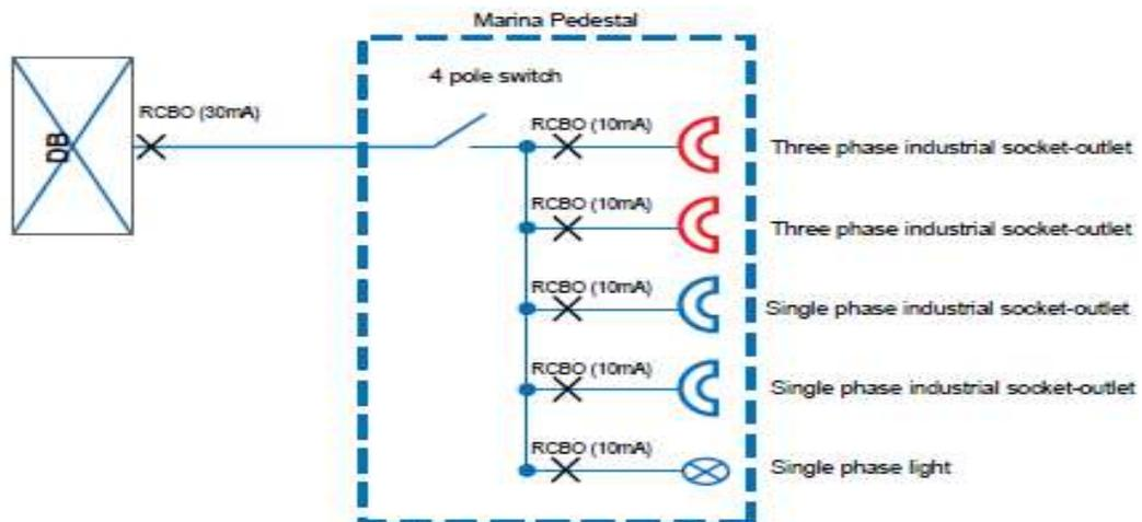
Note 1: protection can be provided by a combination of suitably rated MCBs and suitably rated RCDs.
