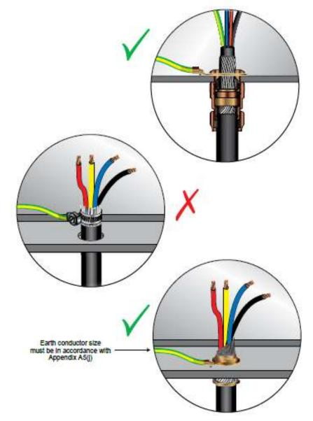
Note: all glands should be mechanically and electrically sound, secured and tightened using the appropriate tools
